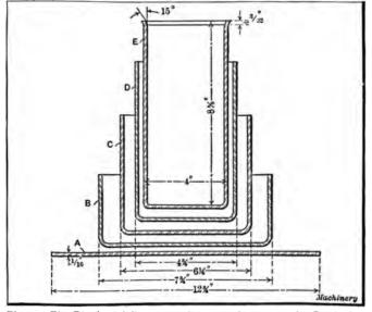
Fig. 4. The Blank and Successive Drawing Operations for Producing Steel Shell E
